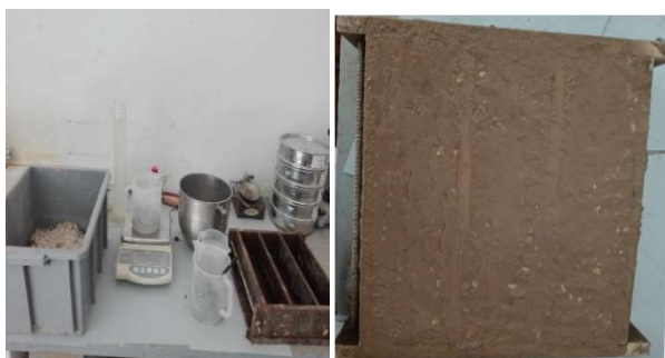
Fig. 3: Instrumentation and mold (7x7x28) preparation
