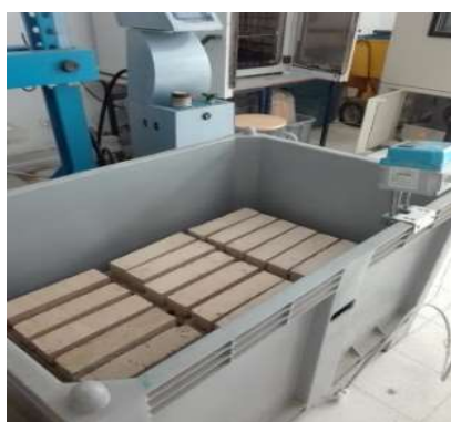
Fig. 4: Moist chamber for conservation of earth blocks.
