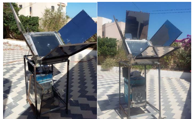
Fig. 6 Solar collector with different reflectors configurations
