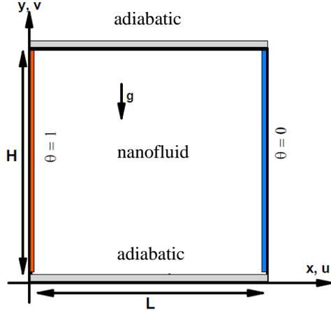
Fig.1: Differentially heated cavity filled with a nanofluid.
