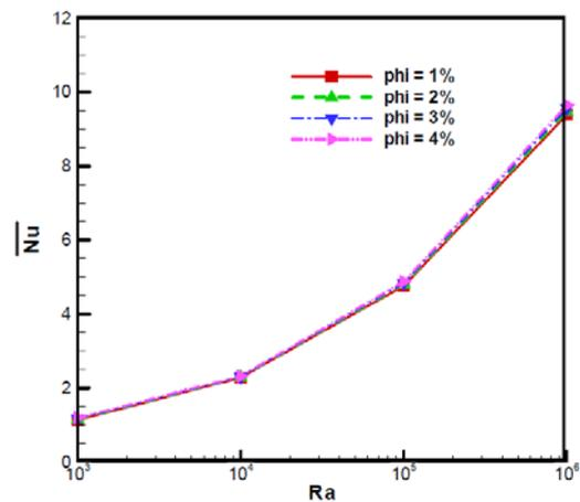
Fig.6 .Variation to the average Nusselt number on alumina according to the concentration of nanoparticles ( $1\% \leq \phi \leq 4\%$ ) and at different Rayleigh numbers ( $10^3 \leq Ra \leq 10^6$ ).
