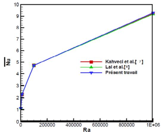
Fig.3 .Variation to the average Nusselt number on water at different Rayleigh numbers in the range  $10^3$ - $10^6$ .
