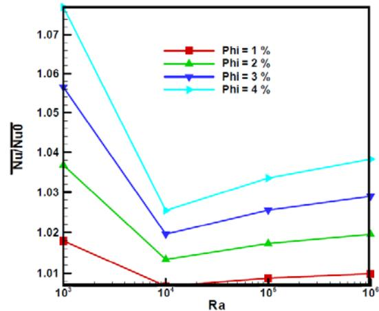
Fig.8 .Profile of the ratio of average Nusselt number on alumina with water according to different Rayleigh numbers in the range 10<sup>3</sup>-10<sup>6</sup> and at different concentrations of nanoparticles in the range 1% ≤ φ ≤ 4%.
