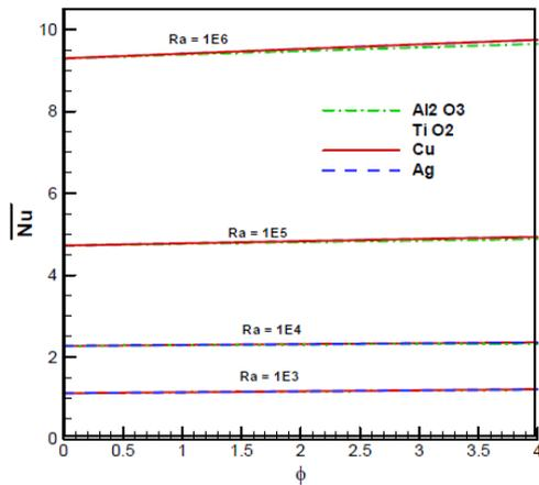
Fig.7 .Profile of the average Nusselt number as a function of the nanoparticle concentration on different Rayleigh numbers in the range 10<sup>3</sup>-10<sup>6</sup> for four different nanoparticles.
