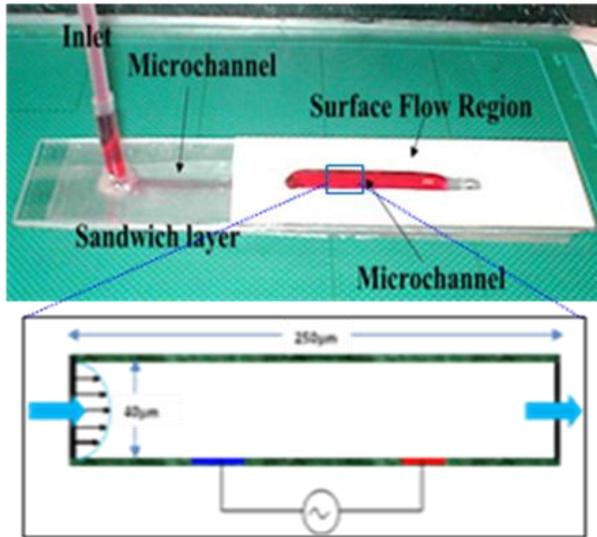
Fig. 1 2D model simulation: a section of microchannel with two electrodes in lower boundary.
