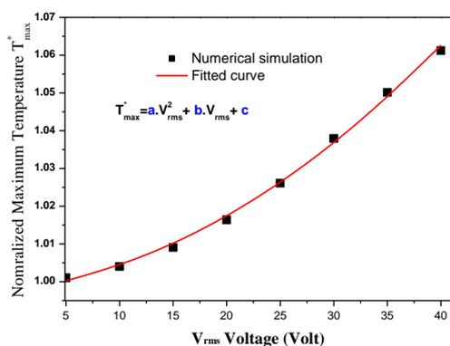
**Fig. 5** Normalized maximum temperature at 15 kHz with the curve-fit.
