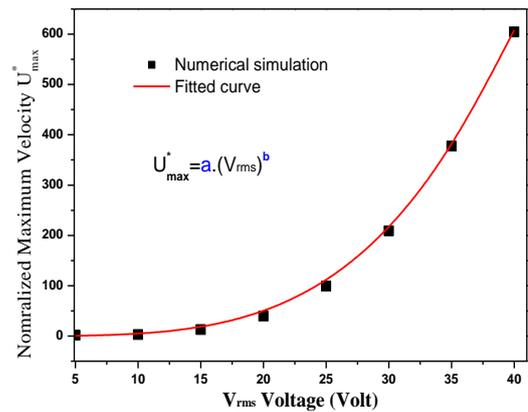
Fig. 3 Numerical simulation result of fluid velocity as a function of the applied voltage at 15 kHz.
