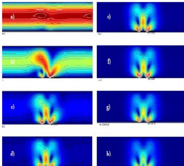
Fig. 2 The distribution of the flow velocity field with 15 kHz for different applied voltage: a) 5V, b) 10V, c) 15V, d) 20V, e) 25V, f) 30V, g) 35V, and h) 40V, respectively.
