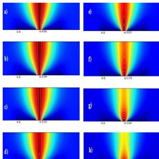
**Fig. 4** The distribution of the temperature field with 15 kHz for different applied voltage: a) 5V, b) 10V, c) 15V, d) 20V, e) 25V, f) 30V, g) 35V, and h) 40V, respectively.
